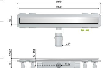
Renova Name Misura-HM 60 Water seal 35 Water volume 33
