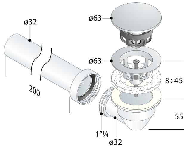
**Misure**  $\varnothing 63 \times \varnothing 32$
